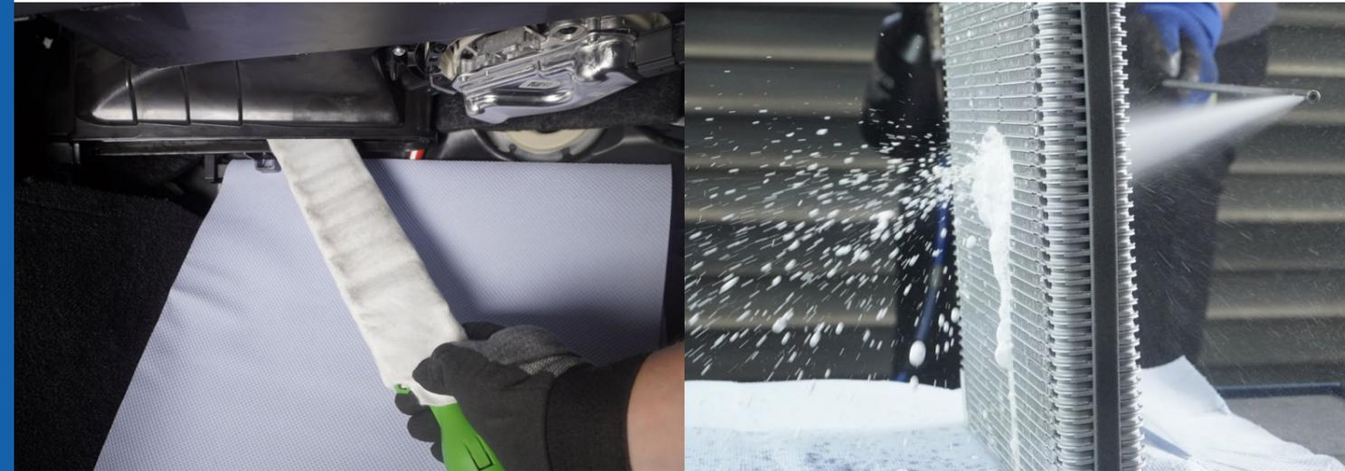
The special **airco well**<sup>®</sup> cleaner for the pollen filter box removes all dirt before inserting a new pollen filter. The housing is wiped free of residue and dirt is removed by using the specially developed cleaning tool and a microfibre cloth soaked with cleaning chemicals. Alternatively, the cleaning aerosol can be spread in the pollen filter box using a spray probe and afterwards wiped out with a microfibre cloth.
