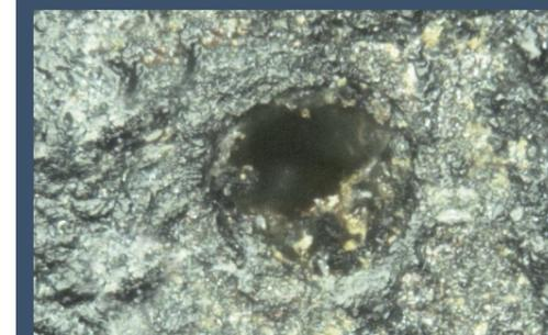
INJECTOR INJECTION HOLE | BEFORE
