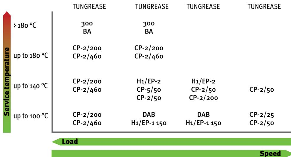
Selection of lubricating greases on the basis of temperature, load, and speed
